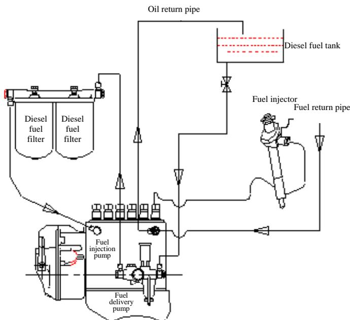
Fig.2-4 Circulation diagram of fuel system
