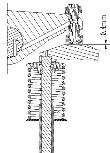
Fig.2-2 Cold state intake valve clearance 0.4mm
