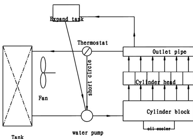
Fig.2-6 Cooling system circulation diagram
