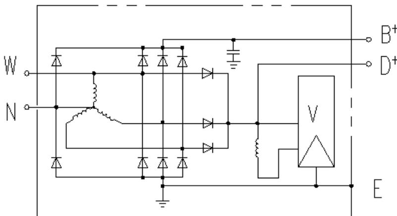
Fig.2-9 Generator circuit diagram
