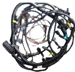
Figure 2-7 Engine wiring harness
