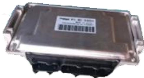
Figure 2-6 Engine control unit
