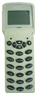
Figure 2-16 Handheld debugger
