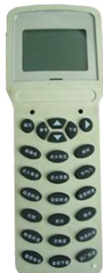
Figure 2-21 Handheld debugger
