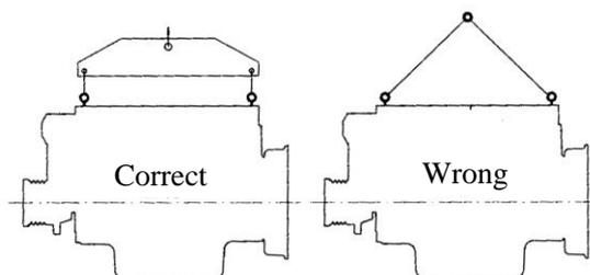
Figure 3-1 Lifting diagram of natural gas engines
