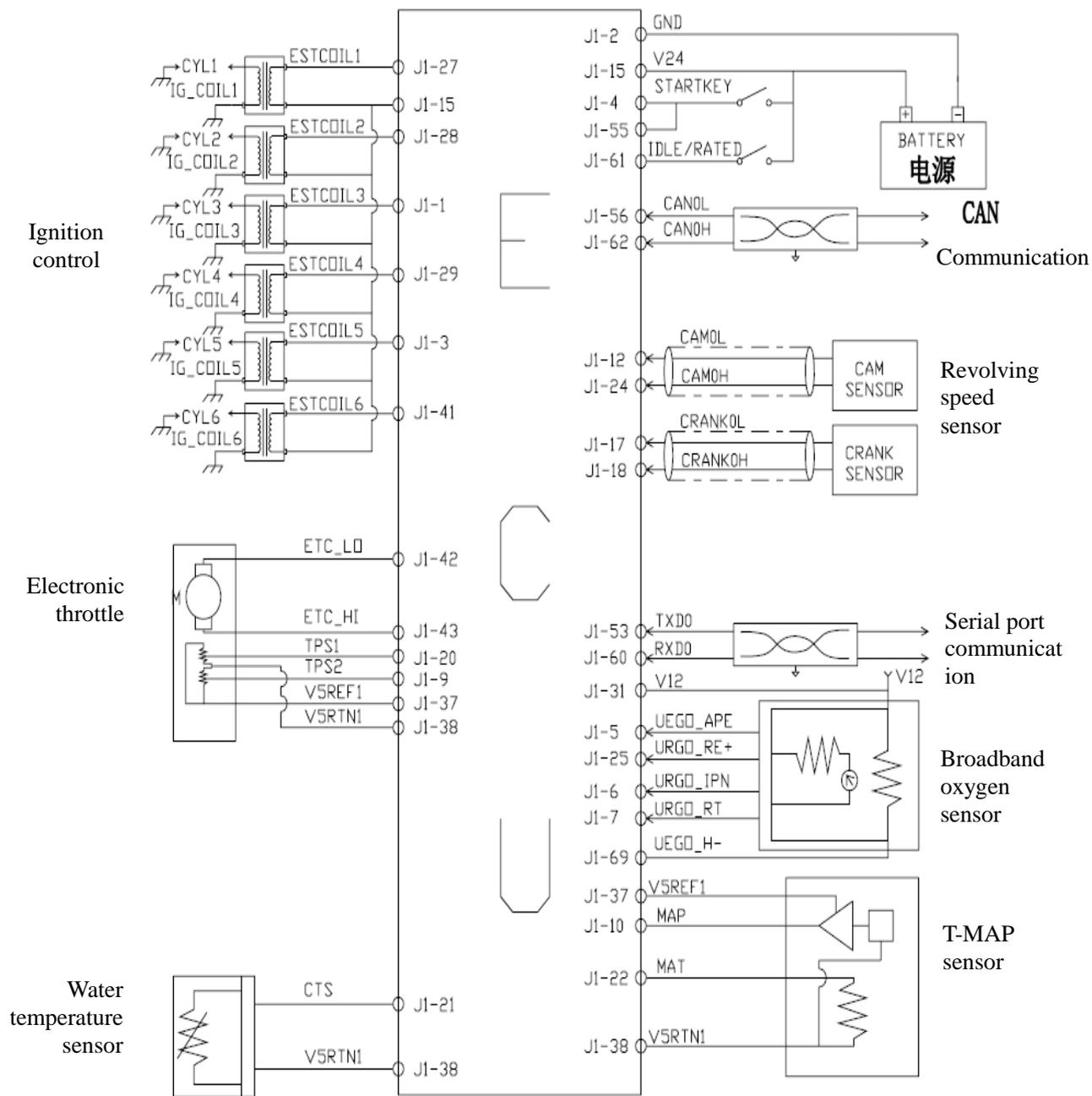
Figure 2-8 Electronic control schematic diagram
